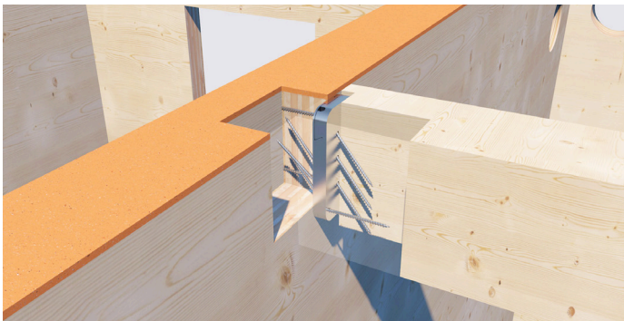
Magnus hook connector for installing a beam on a wall.
